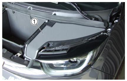
Unlock the plug for high voltage disconnect (1) and pull apart in the direction of the arrow.
