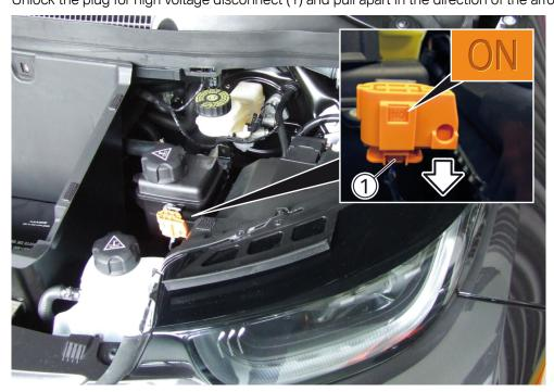
The high voltage system is deactivated when the hole (1) is clear all the way through.
