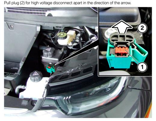
The high voltage system is deactivated when the hole (1) is clear all the way through.
