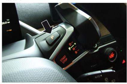
Pull the switch for the electric parking brake upward.
