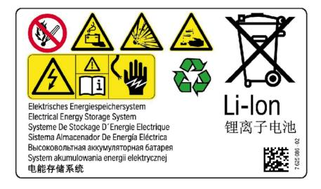
Labelling of the remaining high voltage components:
