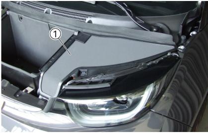
Unlock plug disconnection lock (1) and pull upwards.
