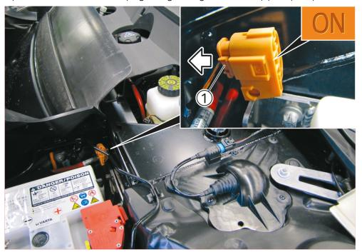
The high voltage system is deactivated when the hole (1) is clear all the way through and the word "OFF" can be seen on the plug.
