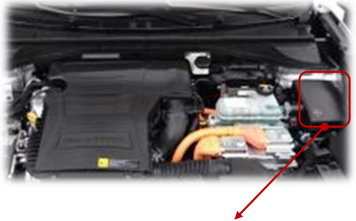
Engine room fuse box
